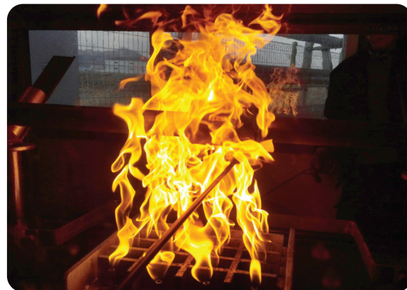
Test Details : A fire resistance test was conducted for 30 minutes at 800°C. (Pressure of 18kgf/cm 2 maintained)
