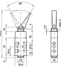
\*Rotation at Point of Application:  $40\,^\circ$  minimum @ 80 mm  $50\,^\circ$  minimum @ 120 mm
