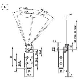
Mechanism may be operated either side of centre line. When the valve is mounted horizontally, the roller is recommended to be positioned on the upper face of the arm.
