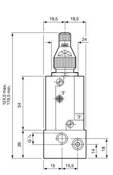
Model Number: M/1430 Port for additional reservoir should remain plugged when not used. Note: Nut used for locking function only, not for panel mounting.
